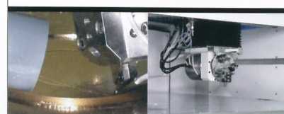
Fresnel lens mold machining Swivel Head (B axis)
