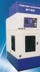
Micro-pattern Imprinting Machine ST50
