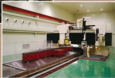
Temperature-controlled factory (Ultra-precision column-type surface grinding machine)
